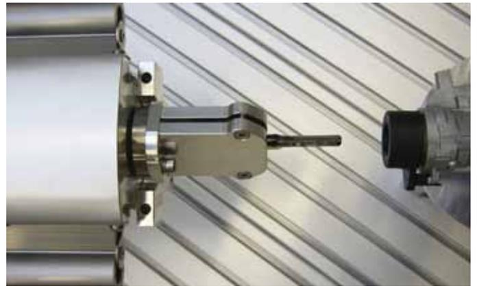
The lock cylinder test bench is made for determining and testing linear forces and torques affecting the vehiclekey and the vehicle lock.
